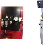
▲ NORTH AMERICAN POWER UNIT / AIR MECHANICAL LOCKING SYSTEM WITH REGULATOR
